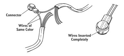
CONNECTING WIRES USING SPLICE CONNECTOR
