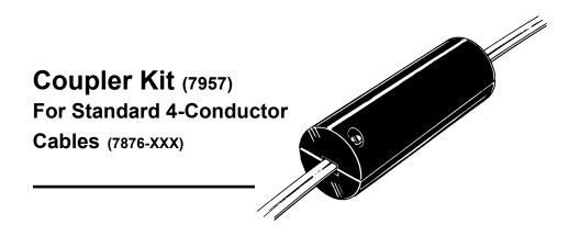
The Coupler Kit (included with Standard 4-Conductor Cables) is used to connect the extension cables to the sensor cables. It includes a cable coupler and waterproof crimp-style splice connectors for making the connection as well as a protective shell in which you may place the connection point.
