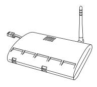
in a field installation. It can be used to free your wireless console from the need to be near the computer, or it can be used in place of either a wired or cabled console. Both cabled and wireless versions are available. Used with our WeatherLink software and data logger, the Weather Envoy allows you to view, store, plot, analyze, export, share, and print your weather data.
