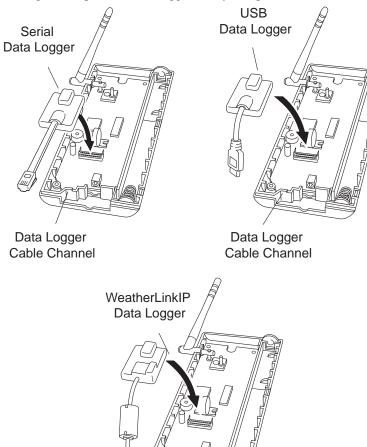
Inserting the Serial, USB or IP data logger into the Envoy
