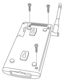
2. Separate the case halves to expose the data logger connector.
