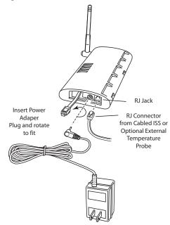
2. Insert the power adapter plug into the power jack.
