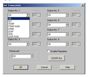
2. Select a Station Type for each of the possible 8 transmitter IDs ("channels") the Envoy may be receiving. See the WeatherLink Online Help System for more information on configuring the stations, the retransmit feature, and configuring the Envoy for using repeaters.
